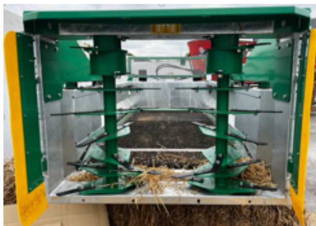
Figure 2. 1: Spread-a-bale internal beater and floor (Source: Authors own)
